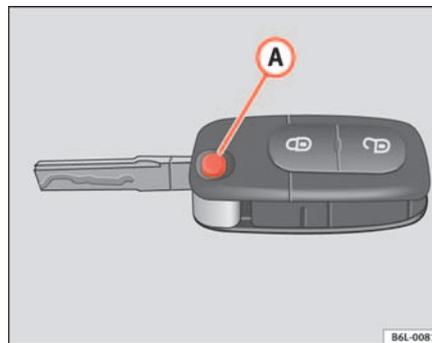
Abb. 56 Klappbarer Schlüssel
