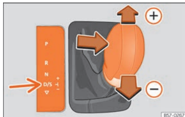
Abb. 88 Hebel in Tiptronic-Stellung.
